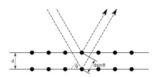
FIG. 1. Bragg diffraction occurs when plane waves with identical wavelengths scatter off adjacent planes of atoms and the path length difference between the two paths is equal to an integer multiple of the wavelength. For electrons, the wavelength is the deBroglie wavelength. Also note that the Bragg angle  $\theta$  is measured with respect to the surface of the crystal.
