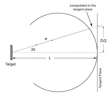
FIG. 4. The geometry of the vacuum tube containing the electron beam, the graphite target, and the fluorescent screen are shown in the figure. In our experiment L is 0.140  $\pm$  0.003 m to the *outside* of the glass, the radius R=66.0 mm, and the thickness of the glass is 1.5 mm.
